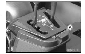
Remove: Quick Rivets [A] (both sides) Seat Lower Cover [B]
